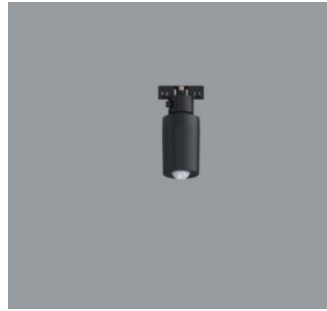
56012.000 ERCO Casambi motion detector with light sensor Black (RAL9011). Setup via Casambi app (Android/iOS) with Bluetooth Low Energy (BLE)-capable mobile devices. Use for daylight-dependent light control with or without motion detector. Detection range of infrared (PIR) sensor 100°/ 5m. At 3m room height, this is a circle with diameter of approx. 7m. Minirail adapter for ERCO Minirail 48V track: polymer, black. Weight 0.05kg CE
